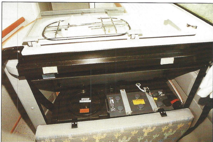
Under the kitchen (with cushion removed) you can see the gas locker (left) and auxiliary battery (right). Waste water tank is also here.
